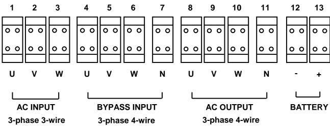
The terminals shown are located at the bottom inside of the 150/225kVA UPS. External cable size is recommended in the Table 1 and 2.
